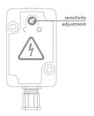
Special care must be taken if the adjustment is made while the power is on. Be sure to use insulated screwdrivers and do not touch anything except the knob.
